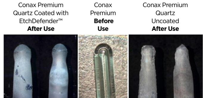
Figure 1. (left) Image of 2 EtchDefender™ TCs run at a Fab in an ASM Epsilon® reactor. (center) Example of the Standard quartz sheath before population with the thermoelements and prior to running in the reactor. (right) Image of 2 Standard TCs run at the same Fab to failure under identical process parameters.
